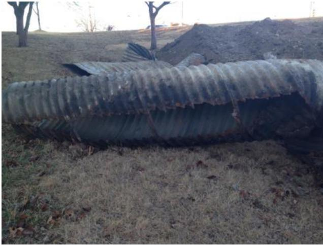
replacement of several hundred feet of pipe, with more to follow in the future. Additionally, an alternative method to replacement is being investigated. This method would involve lining the existing pipe with a cured in place plastic liner, which will eliminate the need to disturb infrastructure (i.e. sidewalks, roads, curbs etc.).
